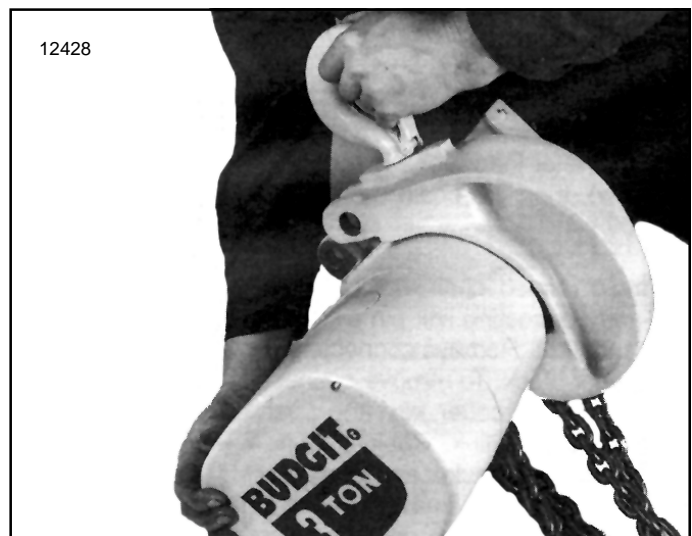
Figure 7-2. Removing 3 Ton Hanger Bracket from Hoist Frame
